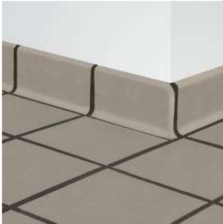
Tile Cove Base installed level with floor tile- NOT on top of floor tile
